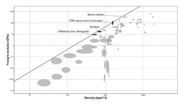
Based on this chart, the ideal candidates for oars are carbon fiber composites or wood. While boron carbide is shown, it would be too brittle.
